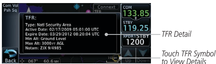
Figure 11-63 Connex TFR Detail
