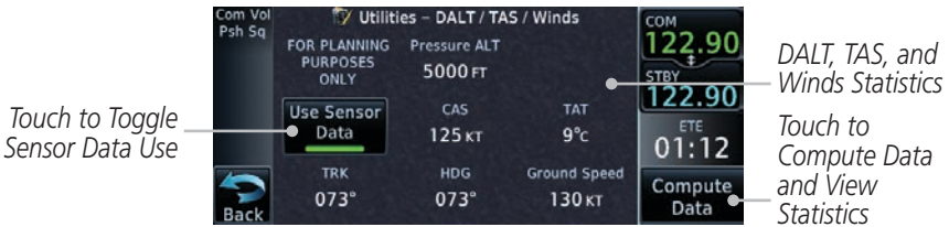
Figure 14-37 Utility DALT/TAS/Winds Page Using Sensor Data and Pressure Altitude
