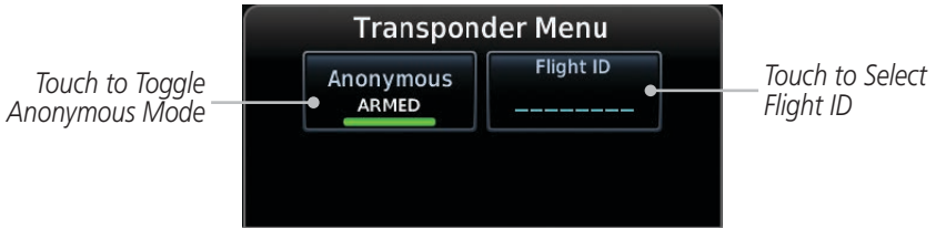
Figure 2-14 ADS-B/Transponder Control Panel
